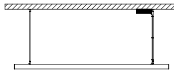
B Suspension installation with surface mounted driver (with canopy).
